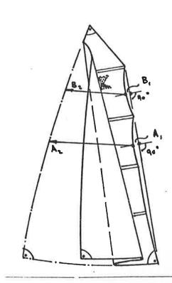
The centre of the clew cringle shall be not more than 40 mm from the boltrope or its extension. No clew outhaul arrangement shall have the centre of its fastening point in the sail more than 40 mm above the boltrope or its extension.
